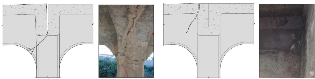
Figure 2: Critical joint failure mechanisms and examples of similar cracking on site
