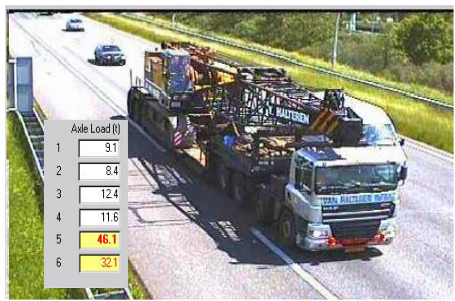
Figure 4: Example critical vehicle captured by WIM (courtesy Rijkswaterstaat, Netherlands).
