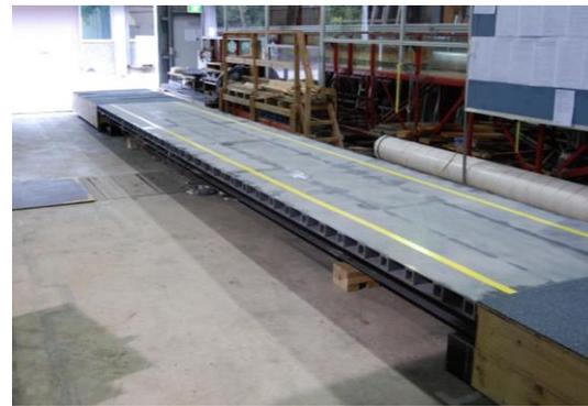
Figure 1 Bonded pultruded FRP footbridge
