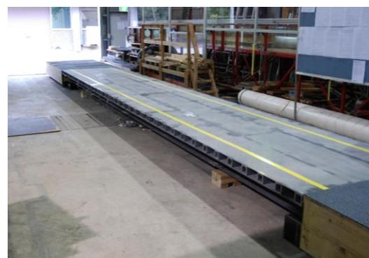
Figure 1 Bonded pultruded FRP footbridge
