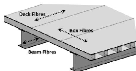
Figure 2 Fibre direction of pultruded FRP members
