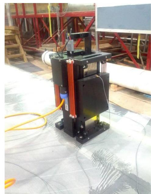
Figure 7 Electrodynamic shaker operating in vertical mode
