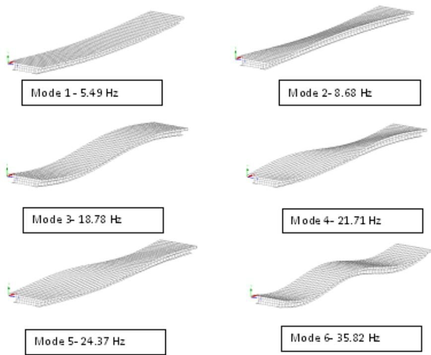
Figure 8 Footbridge mode shapes from FEM
