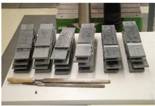
Figure 5 Laboratory testing of bonded FRP plate specimens
