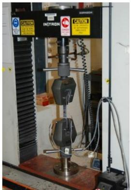
Figure 4 Tensile testing of FRP specimens
