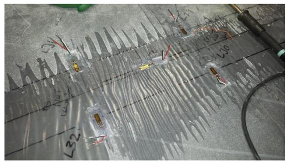
Figure 6 Strain gauges and wiring on deck surface
