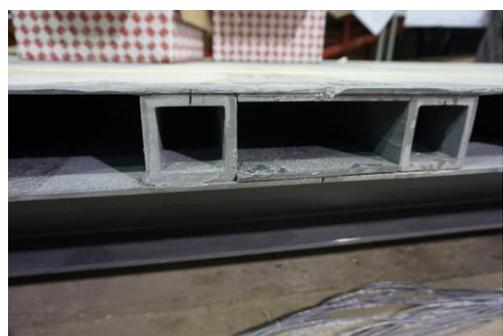
Figure 3 FRP sandwich system as deck supported on FRP I-beams
