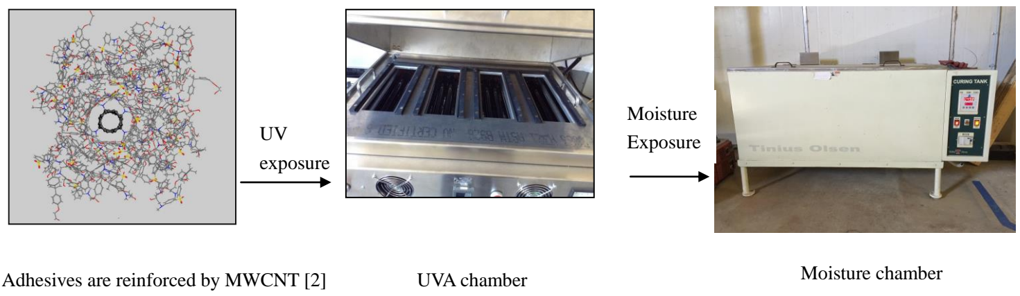
Figure 3: Scheme of artificial accelerated weathering cycle of adhesives during exposure to UV and moisture exposure
