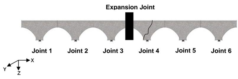
**Figure 1.** Illustration of one of the concrete jack arches underneath the bus lane.
