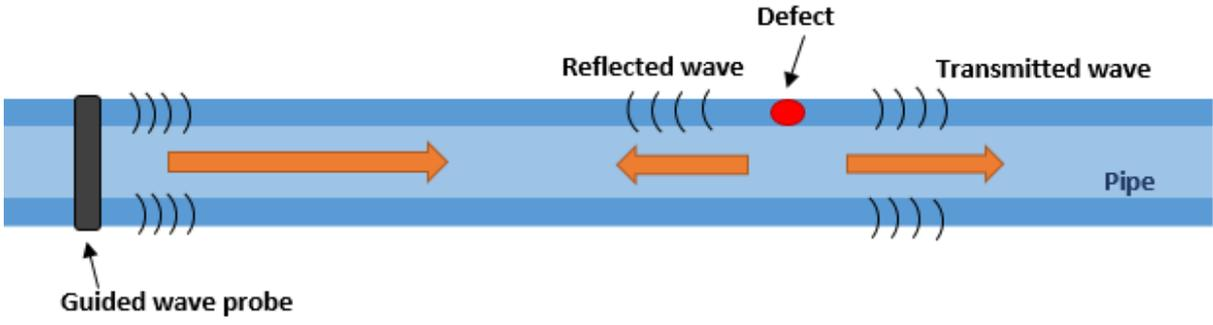
Figure 1 Principle of damage detection in pipes with guided waves
