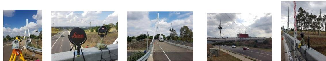
**Fig 5.** Survey targets on bridge.
