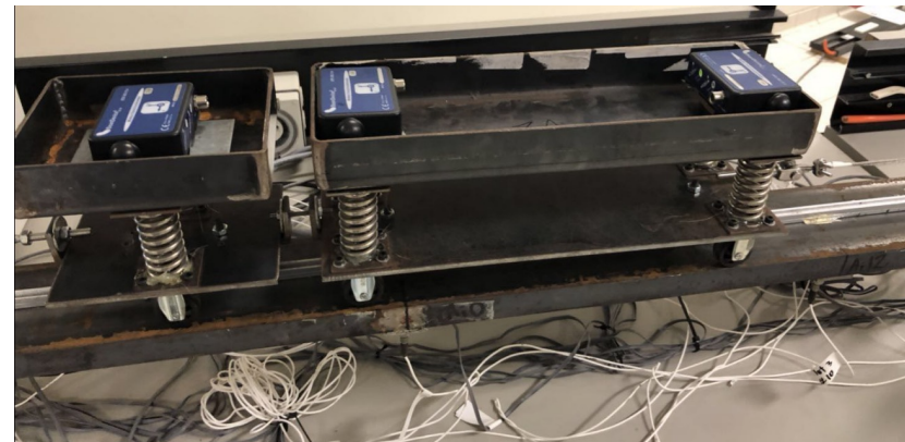
(c) Wireless sensor on the vehicle
