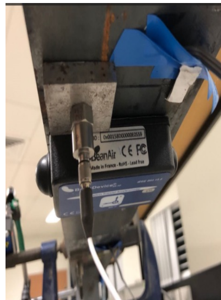
(c) Wireless sensor on the bridge
