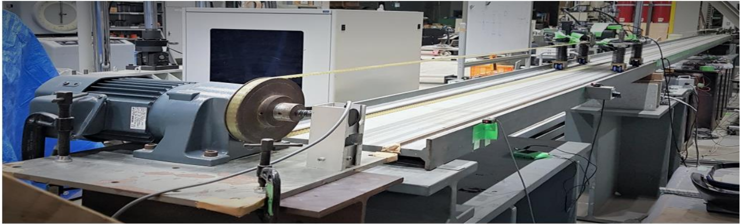
(a) Bridge model, motor and pulley system.
