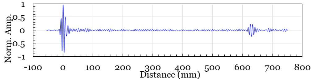
Fig. 3. Detection of a crack-like defect using the  $ES_0$  mode.
