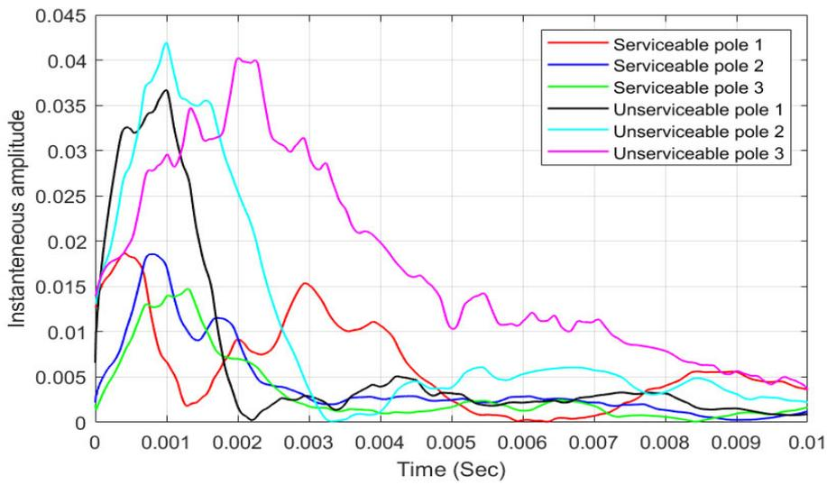
Figure 4. Instantaneous amplitude of IMF1 for AoR2 considering 3 serviceable poles and 3 unserviceable poles.
