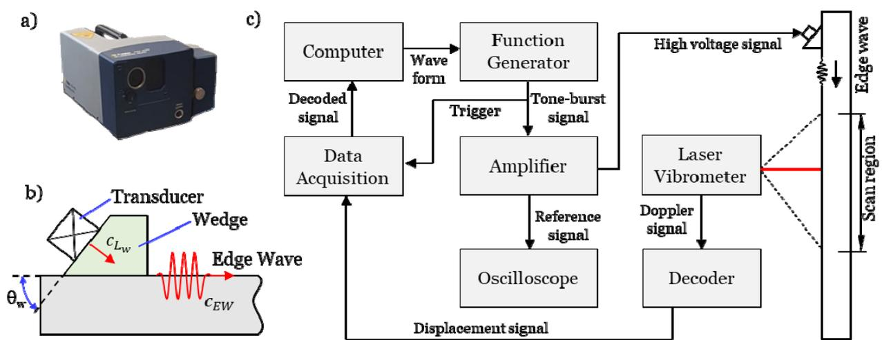
Fig. 2. a) Scanning laser vibrometer head, b) generation of an edge wave using a longitudinal transducer and an acoustic wedge, and c) schematic of typical signal flow and experimental setup
