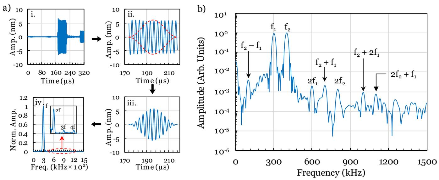
Fig. 5. a) The four main steps in data processing: i. Extraction of the raw displacement signal, ii. Isolation of the edge wave displacement, iii. Application of a Hann-window to the edge wave signal, iv. Results of the FFT, and b) FFT of a frequency-mixed edge wave where  $f_1 = 300kHz$  and  $f_2 = 450kHz$  (these figures adapted from [8] and [9] respectively).
