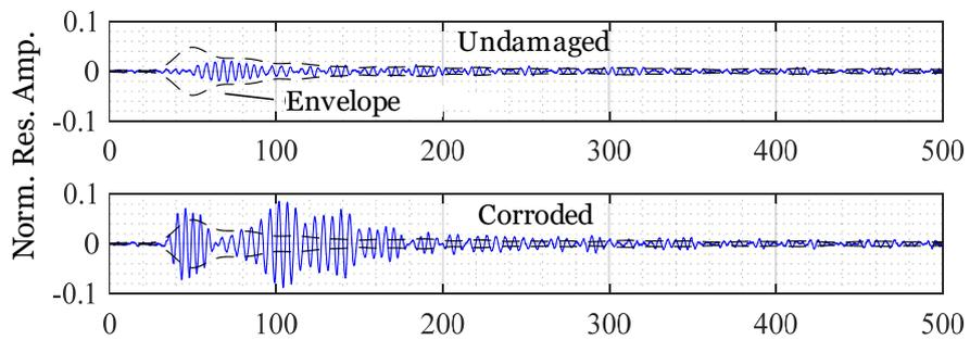
Fig. 4. Detection of distributed corrosion damage using the  $ES_0$  mode and base-line subtraction.
