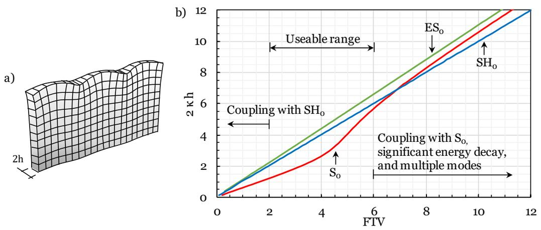
Fig. 1: a) Exaggerated defamations due to edge wave mode propagation in plate of thickness  $2h$ , and b) Dispersion curves for the  $ES_0$ ,  $S_0$ , and  $SH_0$  wave modes.
