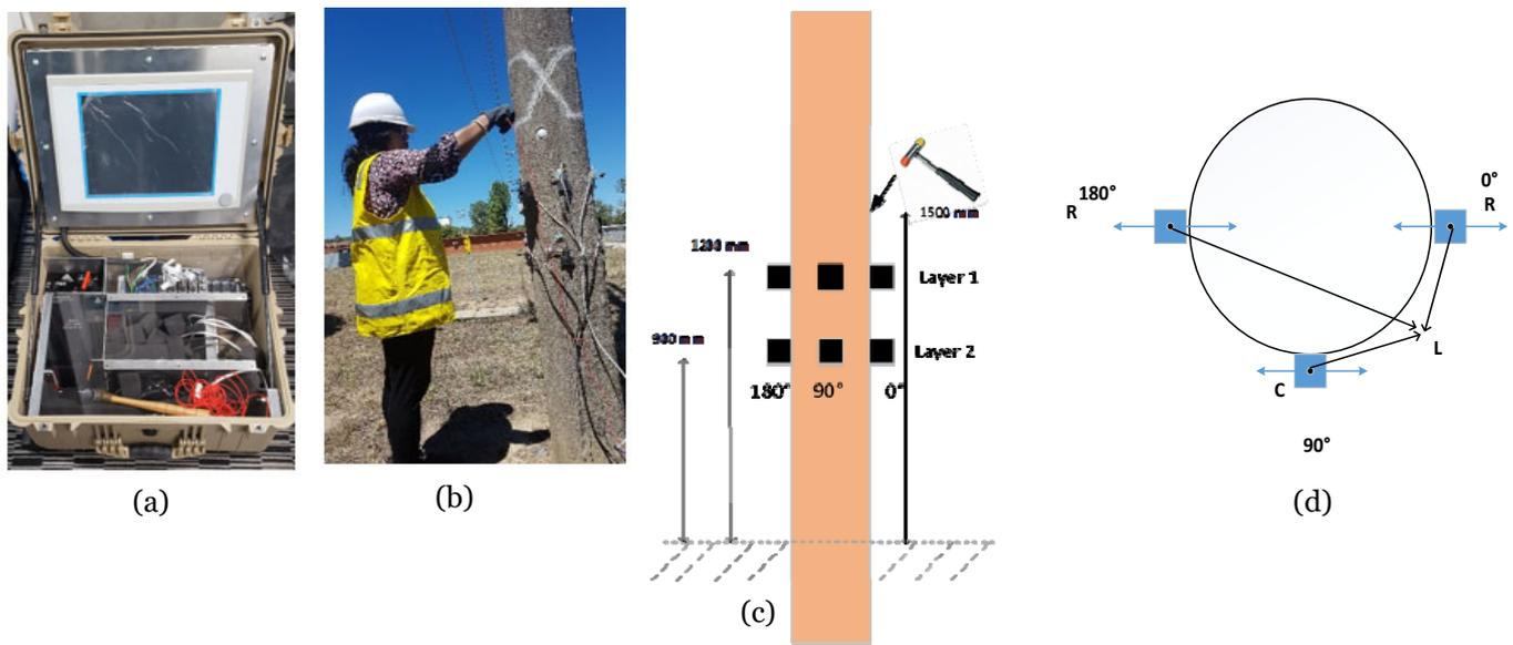
Figure 1. (a) Pole tester (b) Field testing (c) Schematic diagram of experimental test set up (d) Horizontal cross section
