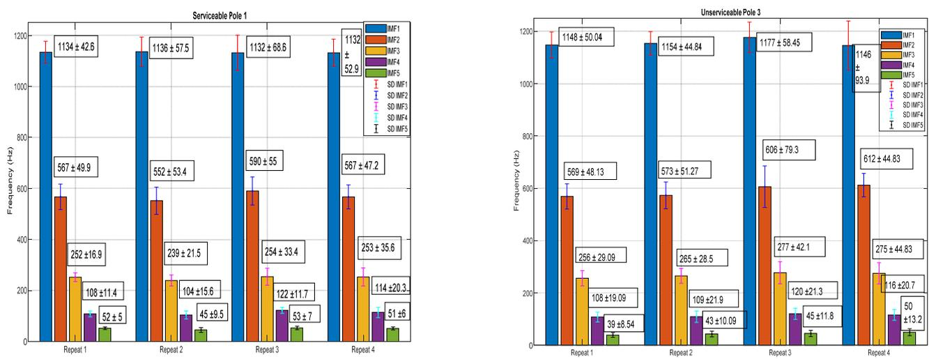
Figure 3: Bar chart showing frequency range of dominant IMFs, average frequency of each IMF and standard deviation for 12 accelerometers, Serviceable Pole 1 and Unserviceable pole 3.
