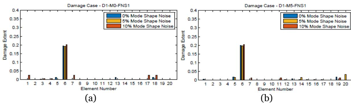
Figure 7: D1-NS-FNS1: Single Damage indices for various Mode Shape Noise and with 1% Natural Frequency Noise;  $\delta\alpha_6 = 20\%$ ; (a) Without mass change and (b) With 5% mass change applied to Element 6
