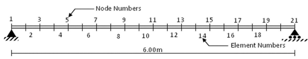
**Figure 2:** Simply supported beam model (adapted from Joseph et al., 2020)
