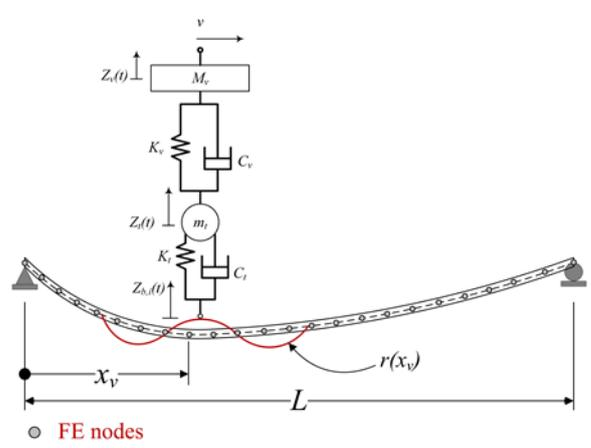
Figure 3 Illustration of the vehicle model.
