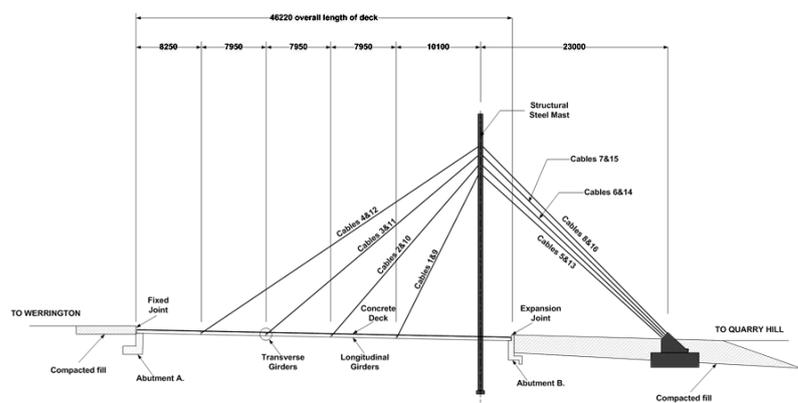
Figure 4 Schematic diagram of the cable-stayed bridge.
