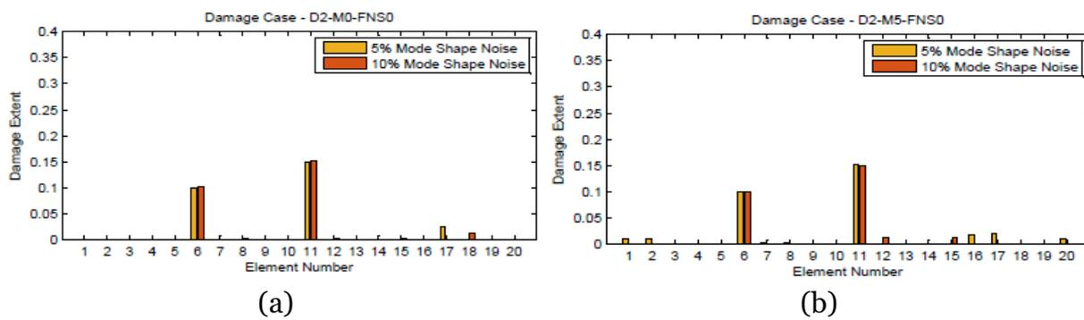
Figure 8: D2-NS-FNS0: Multiple Damage indices for various Mode Shape Noise and without Natural Frequency Noise;  $\delta\alpha_6 = 10\%$ ,  $\delta\alpha_{11} = 15\%$ ; (a) Without mass change and (b) With 5% mass change applied to Element 6
