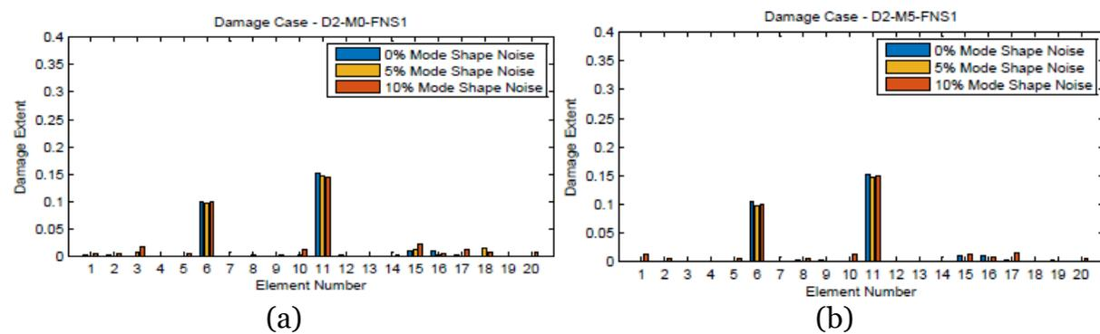
Figure 10: D2-NS-FNS1: Multiple Damage indices for various Mode Shape Noise and with 1% Natural Frequency Noise;  $\delta\alpha_6 = 10\%$ ,  $\delta\alpha_{11} = 15\%$ ; (a) Without mass change (b) With 5% mass change applied to Element 6
