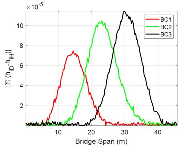
Figure 7 Illustration of damage index obtained for bridge conditions BC1, BC2 and BC3 once vehicle is travelling over the bridge at 5m/s.
