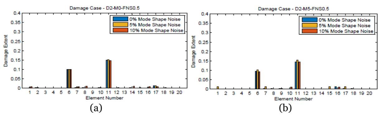
Figure 9: D2-NS-FNS0.5: Multiple Damage indices for various Mode Shape Noise and with 0.5% Natural Frequency Noise;  $\delta\alpha_6 = 10\%$ ,  $\delta\alpha_{11} = 15\%$ ; (a) Without mass change and (b) With 5% mass change applied to Element 6
