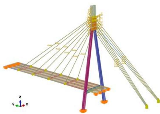
Figure 2 Illustration of FE model of the bridge.
