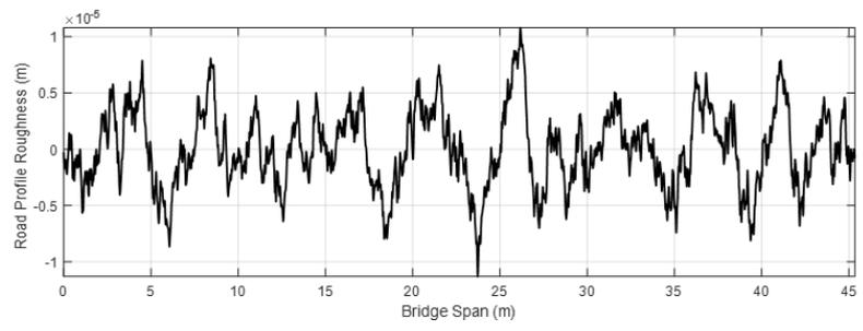
Figure 5 Illustration of road surface roughness with class A.
