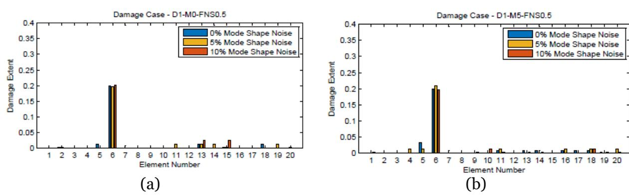
Figure 6: D1-NS-FNS0.5: Single Damage indices for various Mode Shape Noise and with 0.5% Natural Frequency Noise;  $\delta\alpha_6 = 20\%$ ; (a) Without mass change and (b) With 5% mass change applied to Element 6
