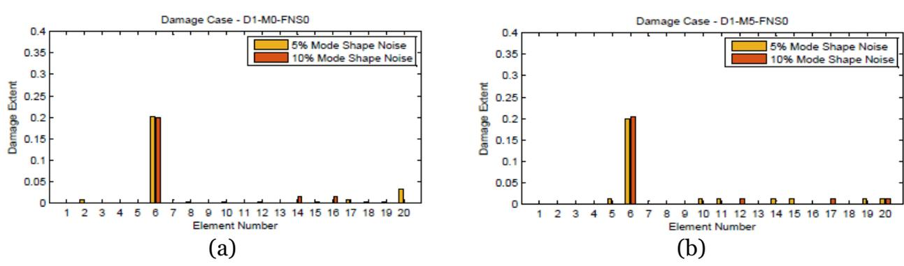
Figure 5: D1-NS-FNS0: Single Damage indices for various Mode Shape Noise and without Natural Frequency Noise;  $\delta\alpha_6 = 20\%$ ; (a) Without mass change and (b) With 5% mass change applied to Element 6
