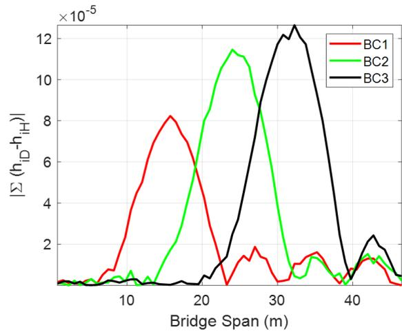
Figure 9 Illustration of damage index obtained for bridge conditions BC1, BC2 and BC3 once vehicle is travelling over the bridge at 15m/s.
