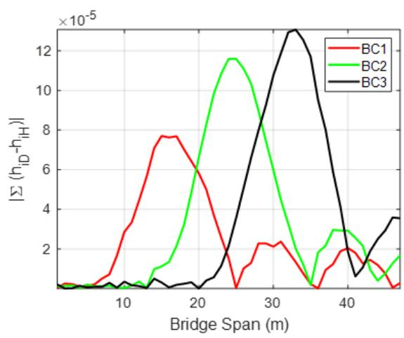
Figure 10 Illustration of damage index obtained for bridge conditions BC1, BC2 and BC3 once vehicle is travelling over the bridge at 20m/s.
