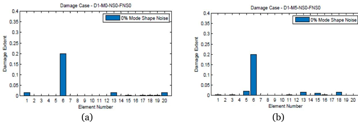
Figure 3: Single Damage indices without Noise;  $\delta\alpha_6 = 20\%$ ; (a) Without mass change (D1\_M0) and (b) With 5% mass change applied to Element 6 (D1\_M5)
