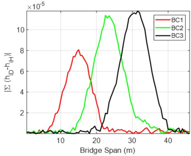
Figure 8 Illustration of damage index obtained for bridge conditions BC1, BC2 and BC3 once vehicle is travelling over the bridge at 10m/s.
