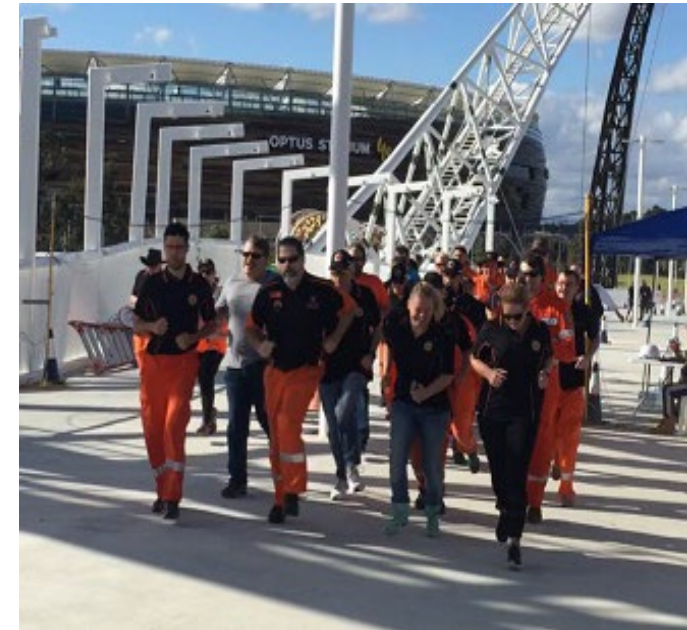
Pedestrians jumping and running on the bridge at a specific pacing rate
