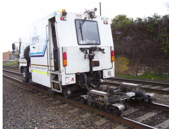
Fig. 1 The ultrasonic testing vehicle
