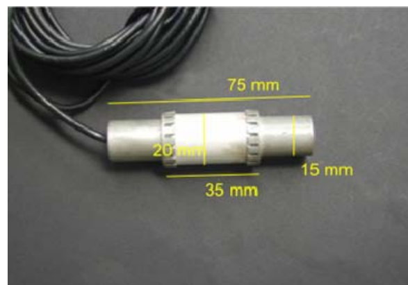
Figure 3. Ultrasonic transducers for embedment in concrete.
