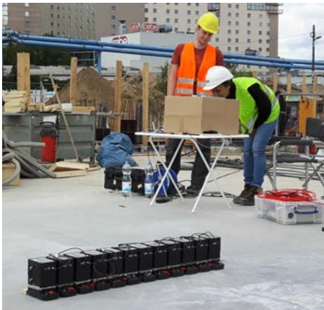
Figure 1. Left: The LAUS applied on a prestressed concrete bridge; Right: SAFT imaging result superimposed to the construction drawing showing the position of the tendon ducts and thickness of the construction.
