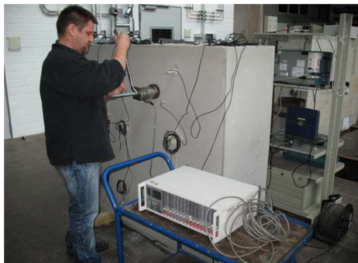
Figure 4. Left: Local load applied to a concrete block monitored by a network of ultrasonic transducers. Right: Decorrelation imaging of the changes in the ultrasonic signal, revealing the area of the block affected by the load; Source: Niederleithinger et al. (2014).
