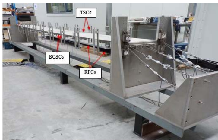
Figure 1. The laboratory suspension bridge model Table 1-Damage Cases
